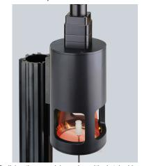
Radial optics open lab version with sketched laser beam. Standard radial optics is closed on sides.
